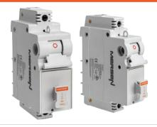
Mersen's Class J Fused Switch incorporates switch functionality with the high protection level of a fuse. The switch accepts UL Class J fuses up to 60A. In addition to this, the Class J Fused Switch is UL 98 listed and suitable for use as main/feeder device and, in conjunction with Class J fuses, is rated for branch circuit protection. It has a smaller footprint compared to a traditional Class J disconnect with a max interrupting rating of 200kA.
